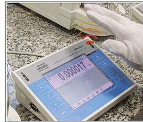
Proximity sensors stand for various ergonomic solutions, they facilitate remote control of functions such as tarring, zeroing, printout.
