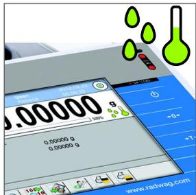
Air pressure, temperature and humidity are parameters measured on-line, signalling system informs when their maximum and minimum values are out of range.
